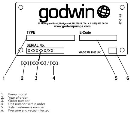
Figure 13: Example of a pump nameplate
