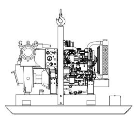
Figure 7: Single lift point skid
