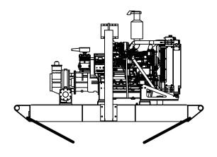
Figure 5: Large skid without D-rings and fork pockets
