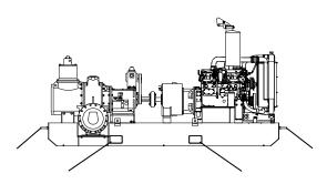
Figure 3: Skid with D-rings and fork pockets
