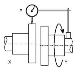
Figure 18: Example of incorrect parallel alignment
