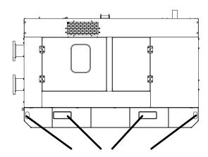
Figure 6: Critically silenced enclosure
