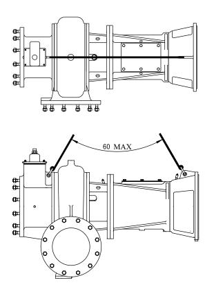
Figure 10: Lift a motor adaptor unit
