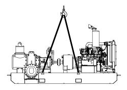
Figure 8: Multiple lift point skid
