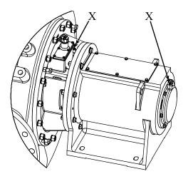
Figure 20: Locations on larger bearing brackets
