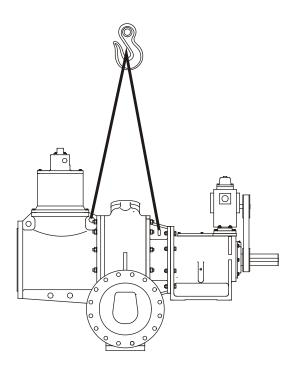
Figure 11: Lift a bearing bracket unit
