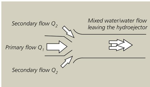
a flushing device. Water ( $Q_1$ ) is pumped through the hydraulic end and out through the ejector pipe, resulting in a powerful jet, which relieves the basin floor and walls of organic matter.
