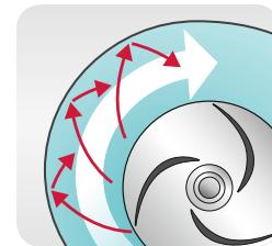
Standard impeller slams solids into the volute.
